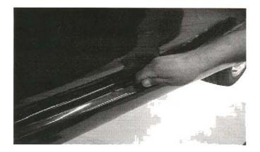
7) Remove side sill panel from vehicle & place in a safe location to avoid scratching.
