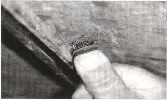
17) Tighten the M5 X 16mm bolt in rear of sill, near front of rear wheel opening.
