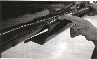
Slide side sill forward until flush with forward section of front sill. Make sure height is even between front & rear sections.
