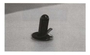
16) Install clips by pushing through side sill & into holes in body. **Note:** The 3 small clips are installed in the front half & 2 large clips in the rear half of sill.
