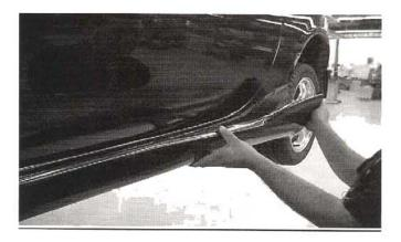
Note: Do not bend or flex panel to avoid damage to paint.
