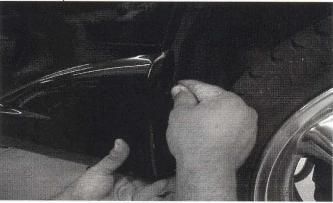
13) Gradually pull plastic backing off of double-sided tape at the same time pushing sill onto body of car.
