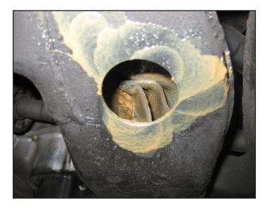
12. Spray undercoating on the underside of the subframe near the four (4) 40 mm access holes and 8 mm drain holes. Do not spray the entire subframe with undercoating.
