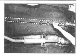
3. On Optima (MG) vehicles, use an air gun to remove debris or contaminants from the fuel tank straps, as shown.
