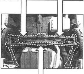
Apply undercoating onto the upper and lower surfaces of the cross member, as shown. Do <u>NOT</u> apply undercoating to the exhaust pipe or other unrelated parts of the vehicle.
