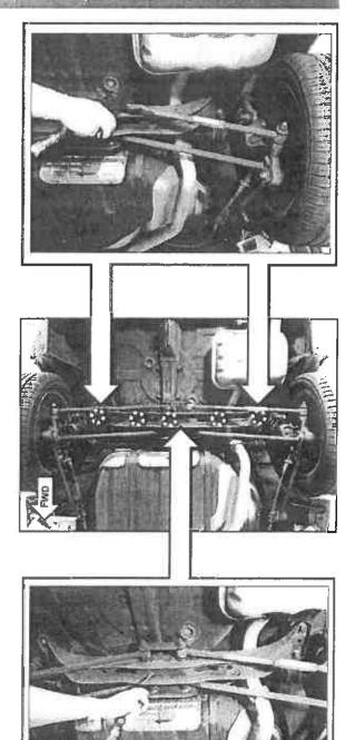
8. Remove any debris from the inside of the cross member using an air gun.
