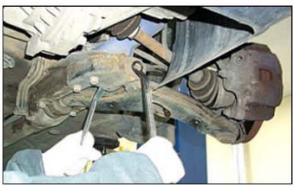
Remove the lower control arm rod bush bracket mounting bolts.
