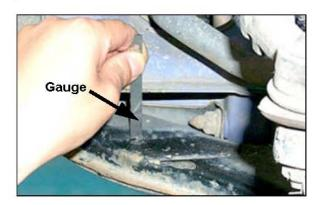
Slide the slit portion in the gauge in the direction of the formed line on the upper panels of both lower control arms to measure the Go/ No-Go thickness at the two arrow locations.
