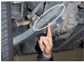
If corrosion perforation or pinholes are observed in any lower control arm as shown, proceed to the "Lower control arm replacement procedure" on page 16 of this bulletin.
