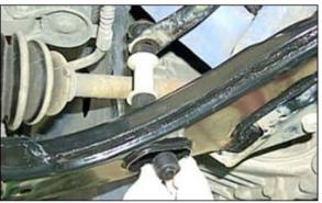
5. Tighten the self-locking nut on the stabilizer link to the specified distance.
