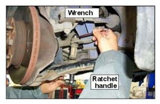
4. Remove the lower control arm bush "A" mounting nut and bolt (17 mm).
