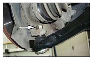
2. Temporarily tighten the left lower control arm bush "A" mounting bolt and rod bush bracket mounting bolts.
