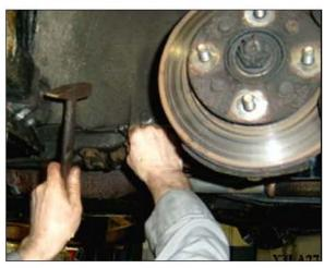
10. Using a center point type 10 mm diameter drill bit, drill the punched points on both sides.
