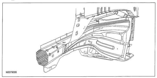
4. **NOTE:** Full frame view. Typical front rail to mid rail section repair.
